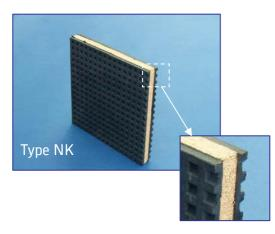
*Type NK Pads* comprises a 12 mm thick cork layer sandwiched between two rubber pads. While not efficient for reducing vibration they have a useful acoustical performance.
