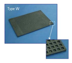
Rubber pads are convenient for reducing vibration and noise in non-critical areas, usually ground floors and basements in applications that do not require the extra efficiency of rubber or spring mounts. They are inexpensive and useful for providing a friction grip that eliminates the need for bolting equipment down.
